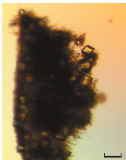
Figure 3 Crystals of boophilin D1 belonging to the orthorhombic space group P2_12_12_1 . The scale bar is 200 \mu\text{m} in length.
